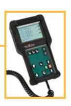
This tethered interface option features larger tactile feedback buttons for the operation of the testing frame; these make it ideal for users who need to wear protective gloves while operating the machine. The display provides simple numerical display of individual channels used on the testing machine.
